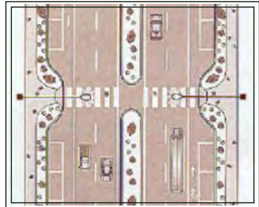
Pedestrian Refuge Island Credit: http://www.safety.fhwa.dot.gov
